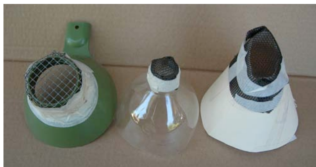
Figure 248. Berlese funnel variations. Left to right: canning funnel with hardware cloth; 2-liter bottle top with pet screen; manila folder with pet screen. “Pet screen” is more durable than regular screen material.
