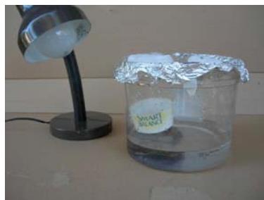
Figure 270. Foil over plastic candy container and goose neck lamp with 100 W. incandescent bulb.
