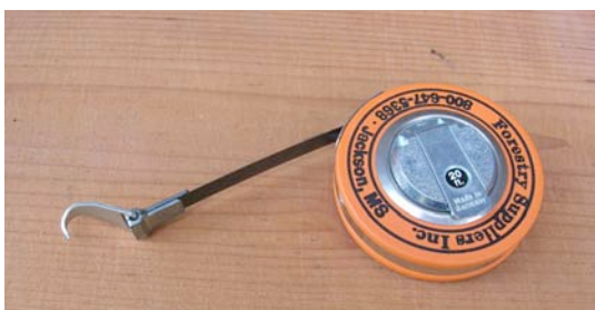
Figure 237. Commercial diameter tape. The hook on the end is placed into the bark to hold the end while the user wraps the tape around the tree.
