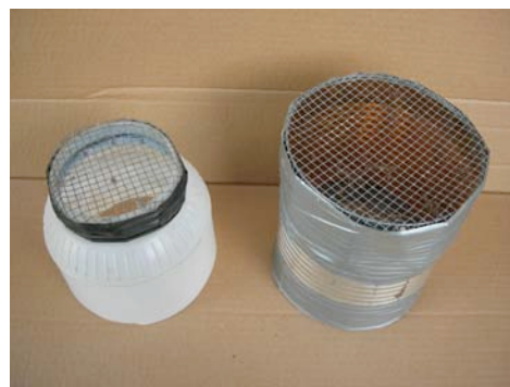
Figure 246. Litter sifters made from plastic gallon jar and #10 can. (Both are upside down and have the bottoms removed.)
