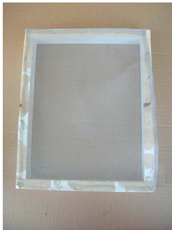
Figure 255. Deckles can be made from scrap wood. A screen shop may donate screen material.
