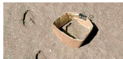
Figure 253. Cardboard strip and binder clips to make "dam" for Plaster of Paris.
