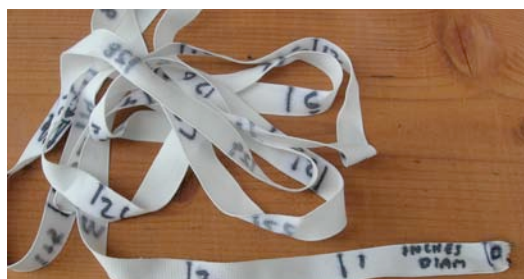
Figure 238. Home-made diameter tape. The end of the tape has been heated to prevent unraveling.
